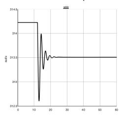
Figure 8. Frequency of the system where the WT contribute to frequency control through pitch deloading strategy.
