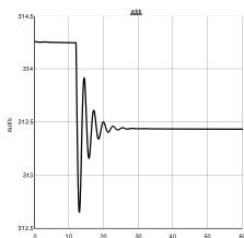
Figure 6. Frequency of the system where the WT does not contribute to frequency control.
